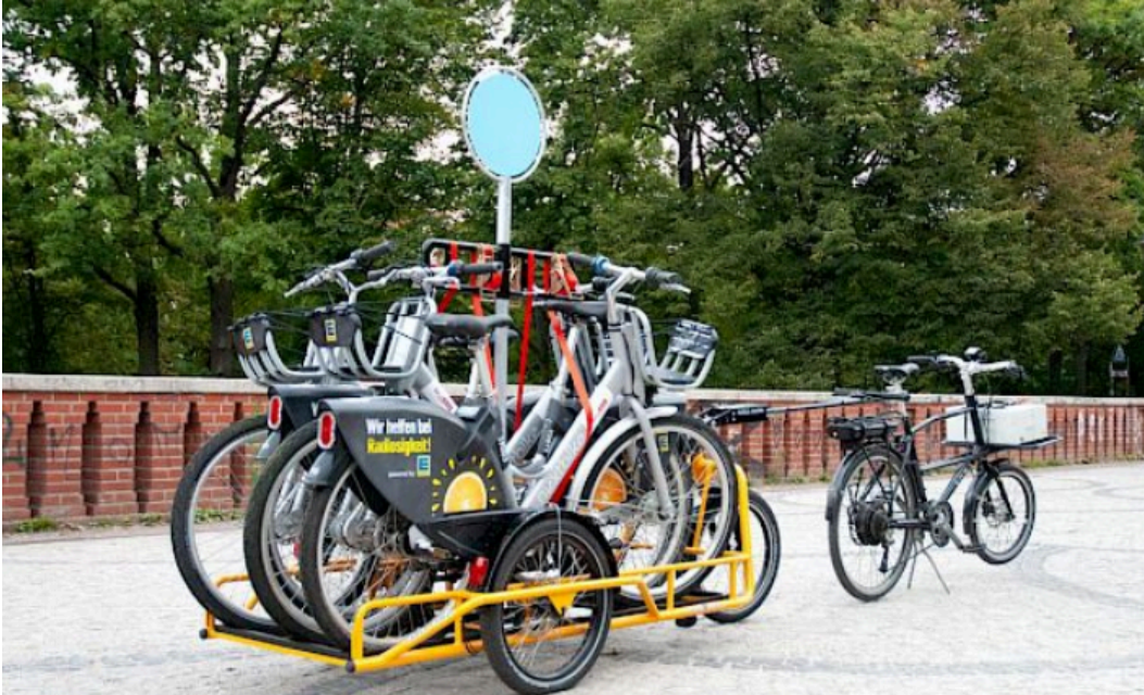
Carla E trailer with bike hauling insert (Video: Carla: See it in action )
